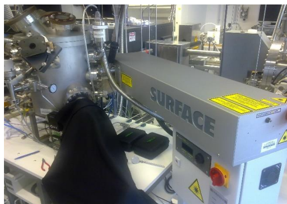
Fig.1: CO 2 laser heater installed at a PLD system
